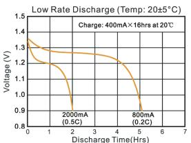
Type: Rechargeable Nickel Metal Hydride Cylindrical Cell
